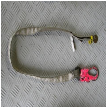
Image 4: Example of Equipment Strop
