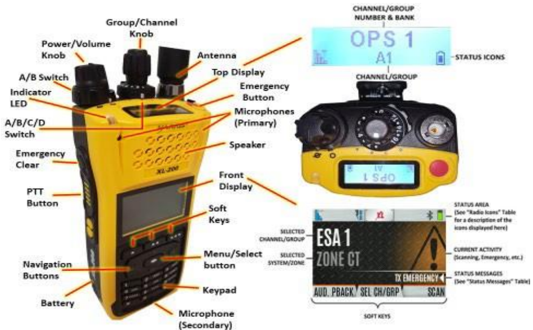
XL – 200P HARRIS RADIO CONTROLS (TOP/FRONT/SIDE VIEWS)
