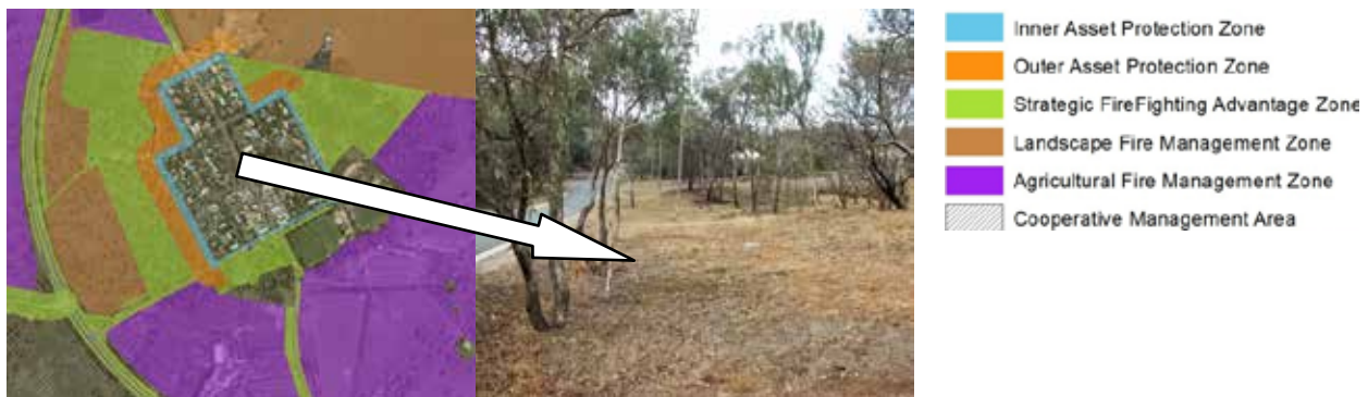
Figure 12 – Hall Village Fire Management Zones, with the photo showing the Inner APZ
